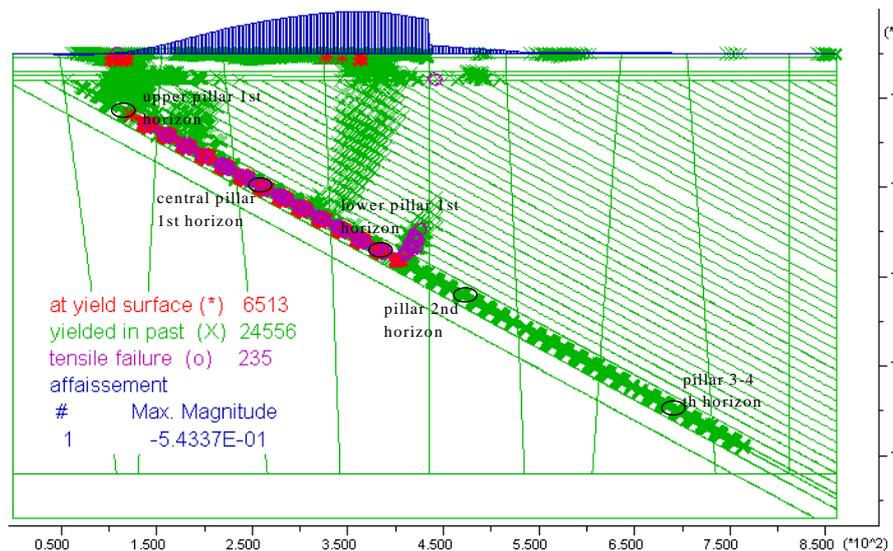
Figure 5: Distribution of plasticity: joint spacing of 10 m + variation of subsidence on the surface
