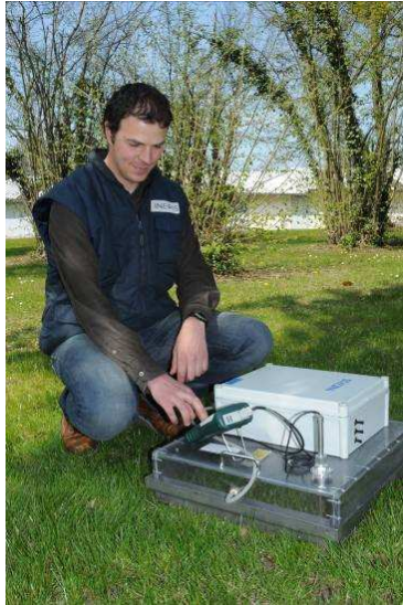
Fig. 1. Performing gas flux measurements at soil-atmosphere interface using an accumulation chamber
