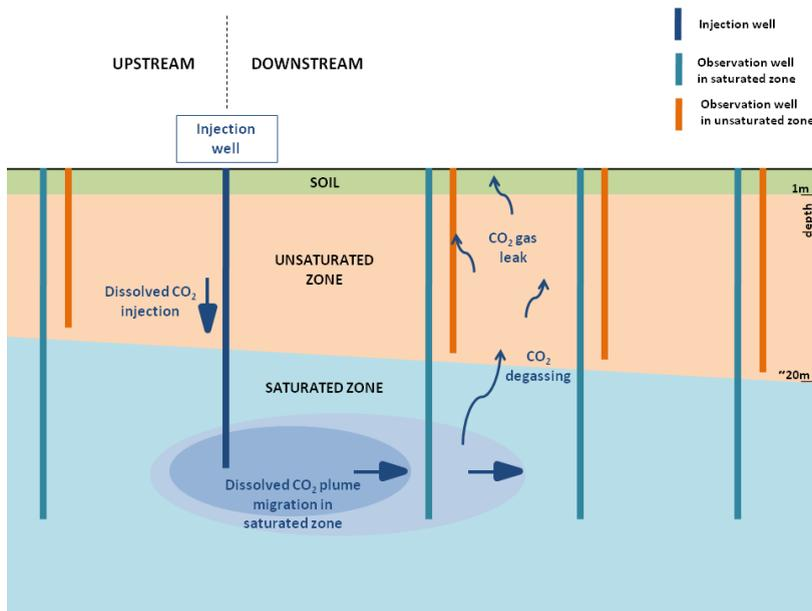
Fig. 6. Pilot site of CIPRES to study impacts of CO<sub>2</sub> leak on subsurface water resource and CO<sub>2</sub> migration and accumulation processes in vadose zone
