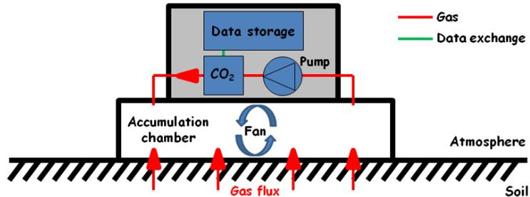
Fig. 1. Performing gas flux measurements at soil-atmosphere interface using an accumulation chamber
