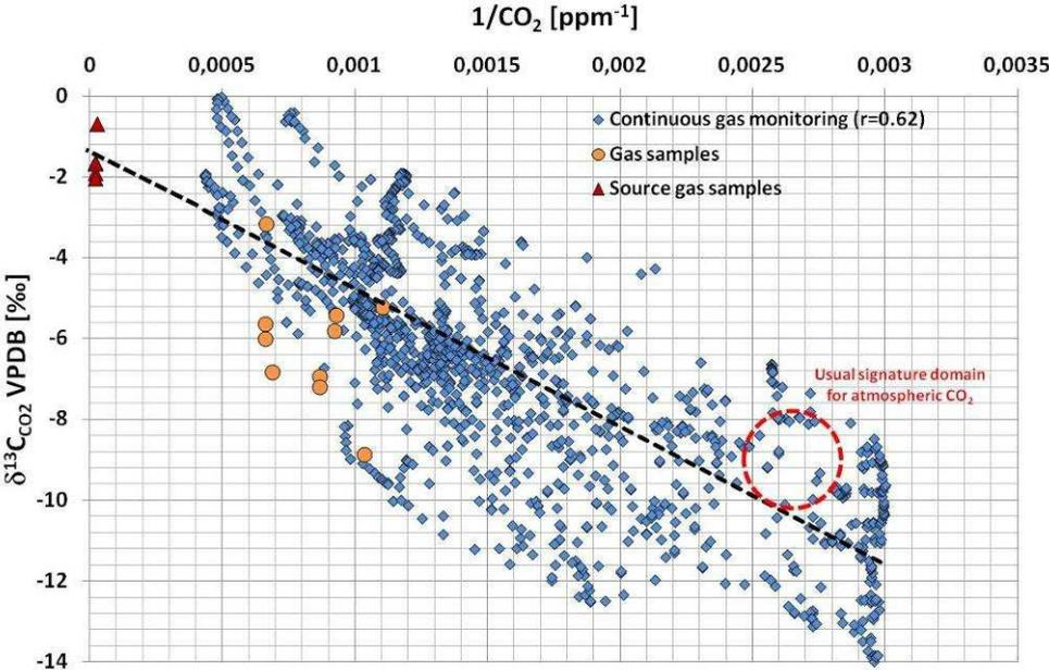
Fig. 4. Plot of carbon isotopic signature of CO<sub>2</sub> gas versus inverse of CO<sub>2</sub> gas concentration (monitored gas appears to be the result of a mixing between atmospheric gas and source gas enriched in CO<sub>2</sub> and having a carbon isotopic signature which is characteristic of a carbonates dissolution process)
