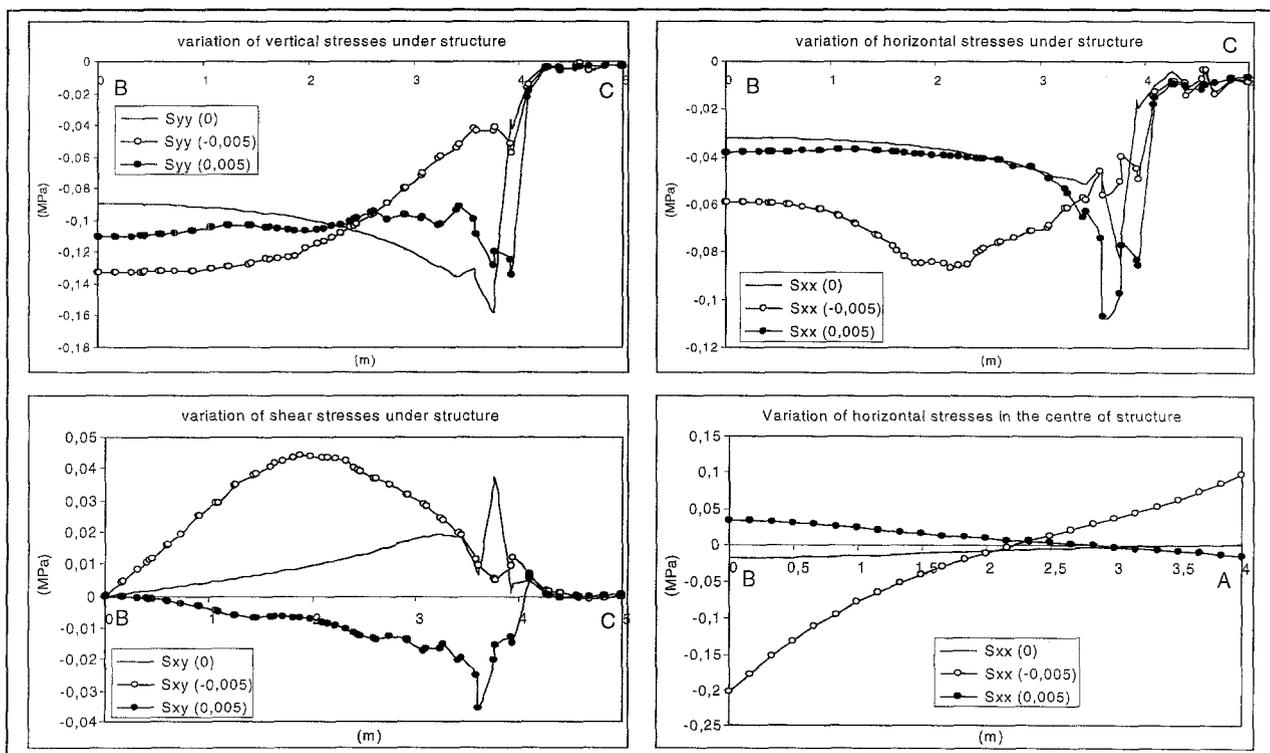
Figure 16 : Stresses along a horizontal section under the structure and along a vertical section in the centre of the structure in a strain area (+/- 5mm)
