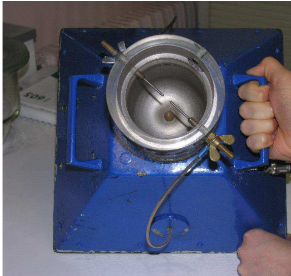
Figure 1: View of the low bottom part of the HARTMANN apparatus (electrodes and dispersion mushroom) on the top of which the Plexiglas tube is settled prior to a test.
