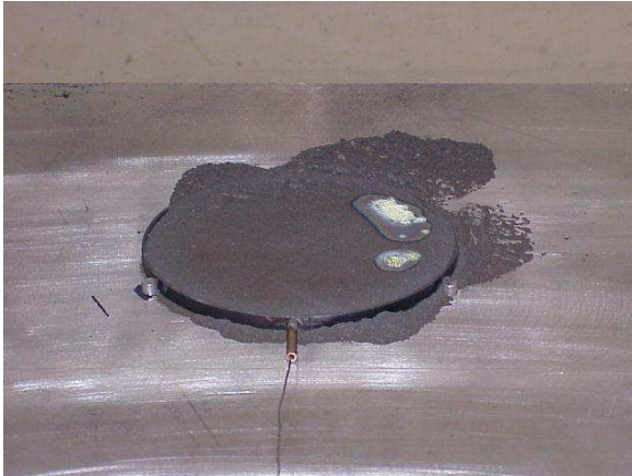
Figure 3: View of the ignition of a 5 mm metallic dust layer during a self-ignition test.
