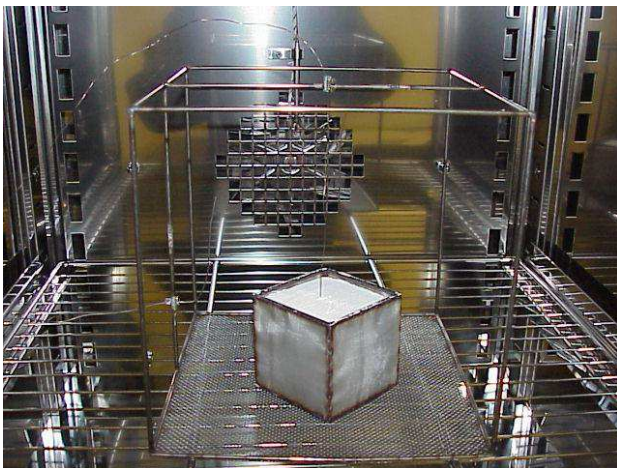
Figure 4: View of a filled basket inside a heating oven.
