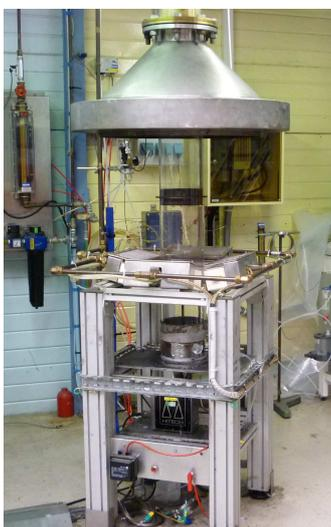
**Figure 1.** The Fire Propagation Apparatus
