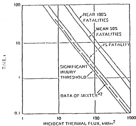
Fatality levels for thermal radiation (Eisenberg *et al.*,<sup>44</sup>)
