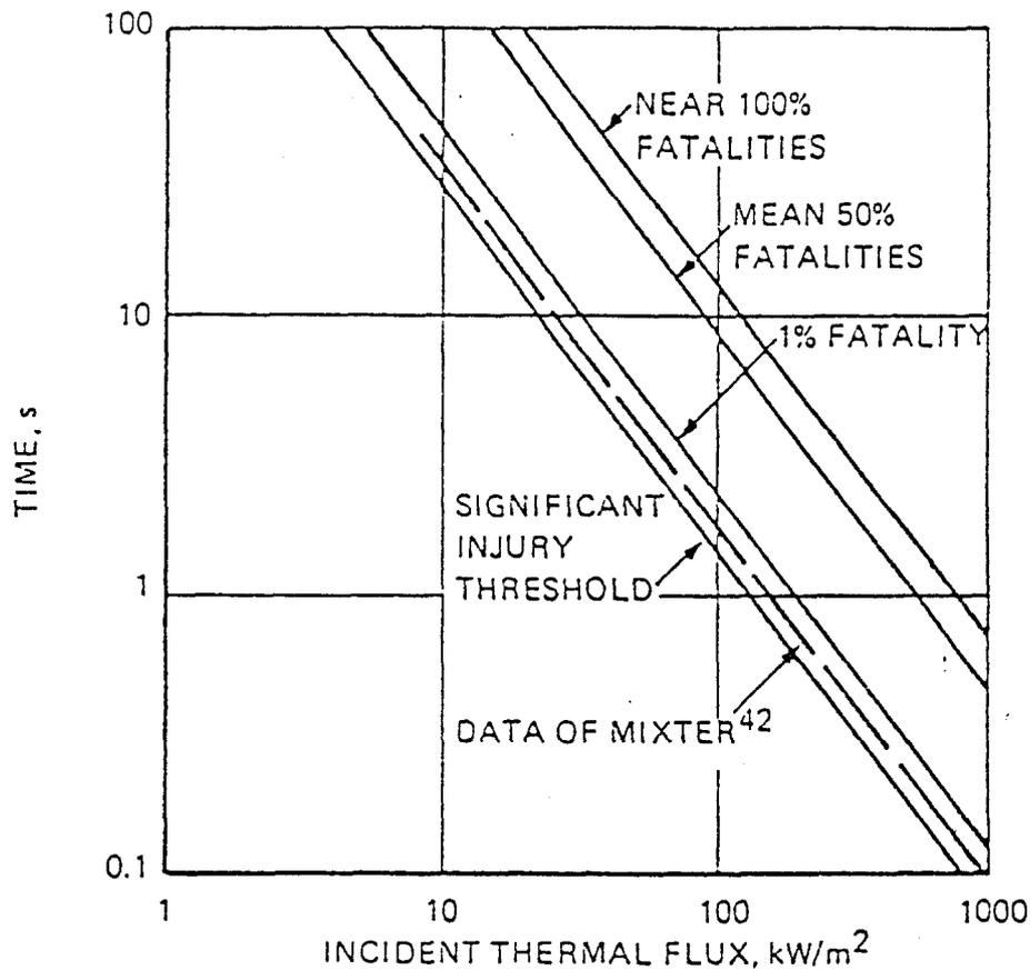
Figure 2 : Fatality levels for thermal radiation (Eisenberg and al.<sup>43</sup>) [From MUDAN (9)]
