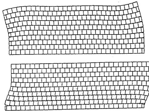
Figure 5. Effects of a shear wave only
