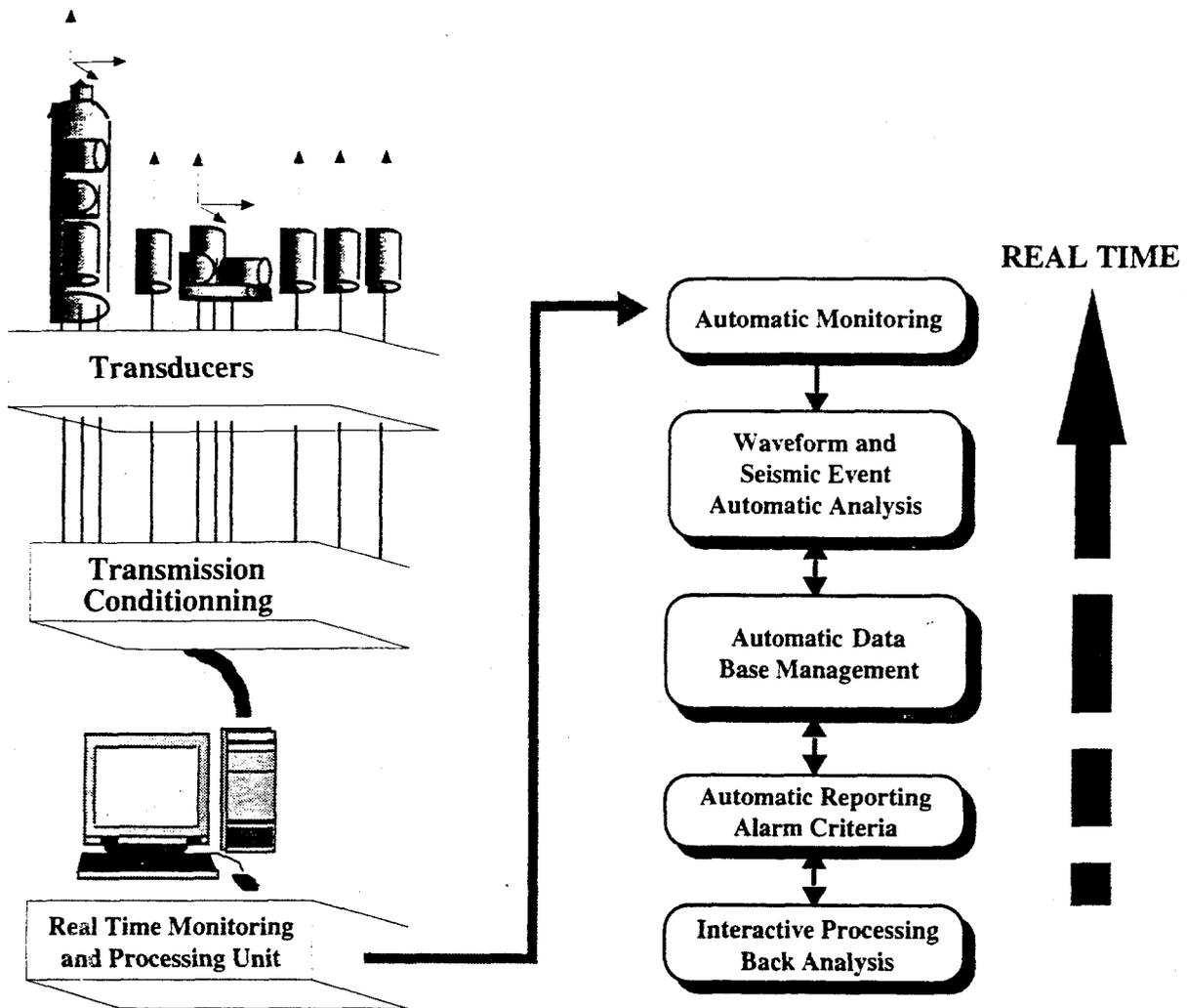
fig. 2 : microseismic monitoring applied to rock failure prevention or back-analysis : high quality, real time systems must handle automatic reporting including last event occurrence analysis, large sequences preceding and 2D/3D mapping based on proper, triggering criteria defined for the area of interest.
