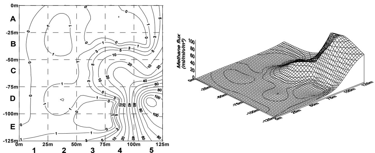
Figure 12. Mapping of methane emission obtained by kriging
