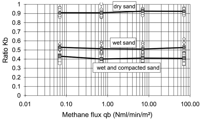
Figure 5. Relationship between ratio  $K_b$  and methane flux
