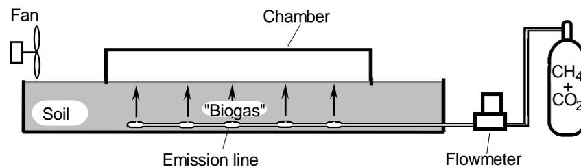
Figure 4. Diagram of test bench for chamber validation
