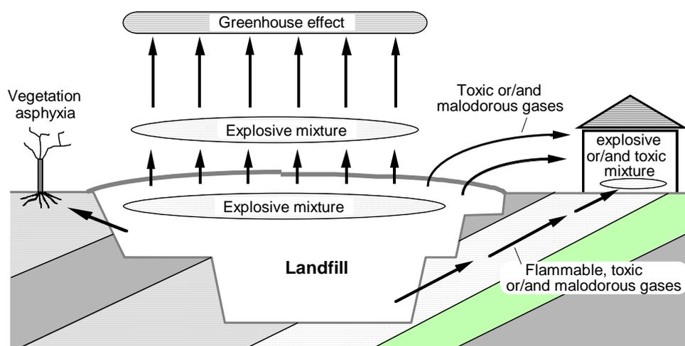
Figure 1. Some forms of potential impact of biogas emissions from landfill
