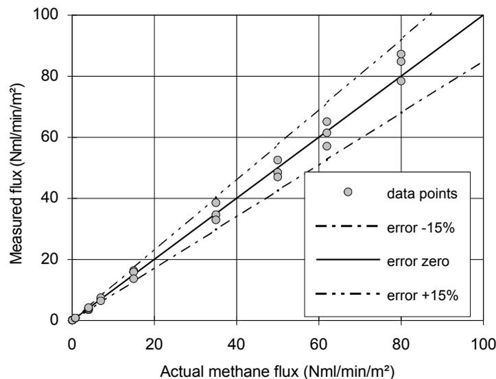
Figure 7. Laboratory results of method reliability test
