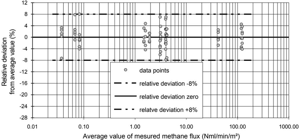
Figure 10. Results of *in situ* repeatability test
