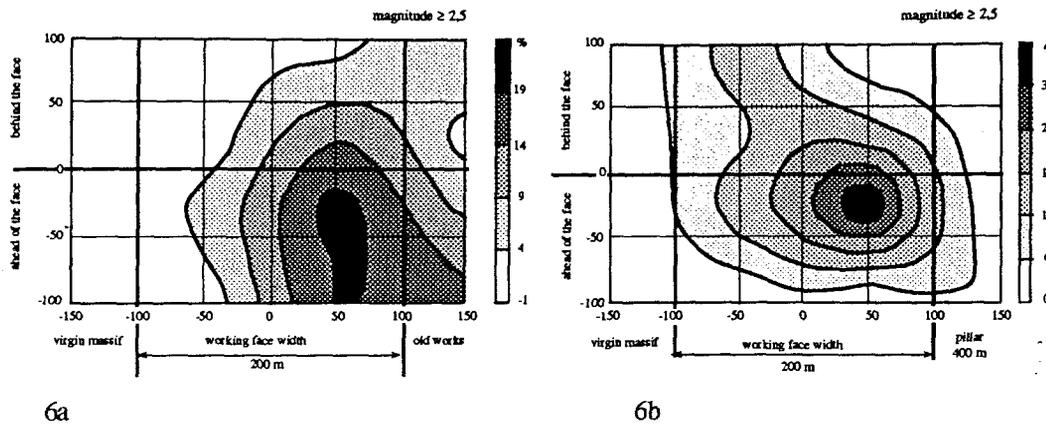
Figure 6: Preferential location of small seismic events (magnitude  $\geq 2.0$ ) induced in the course of operation of working face 07 at the North Estaque district, according to two separate operation configurations: a. geometry 1; b. geometry 2.
