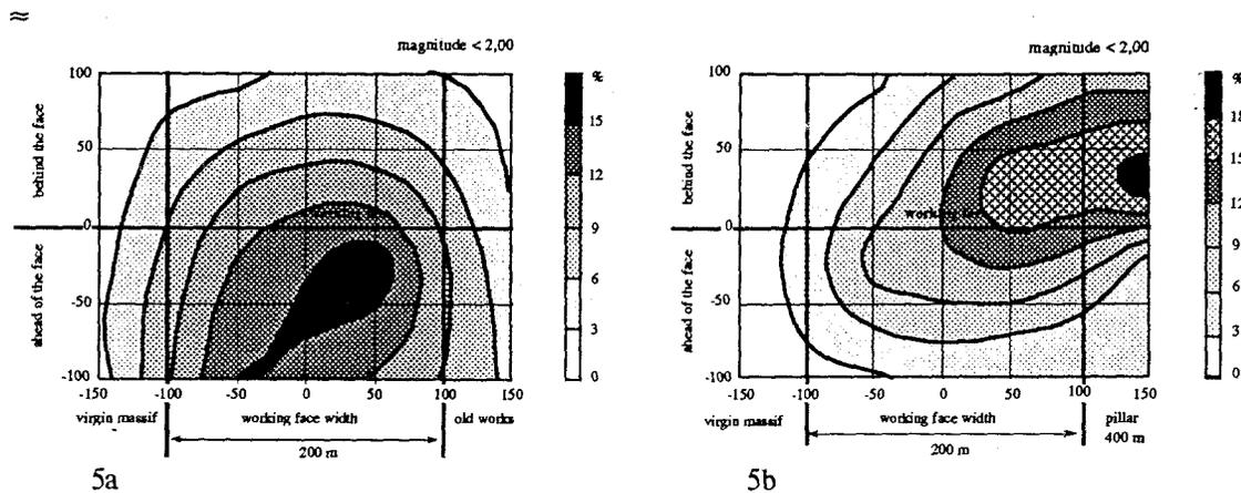
Figure 5: Preferential location of small seismic events (magnitude < 2.0) induced in the course of operation of working face 07 at the North Estaque district, according to two separate operation configurations: a. geometry 1; b. geometry 2.
