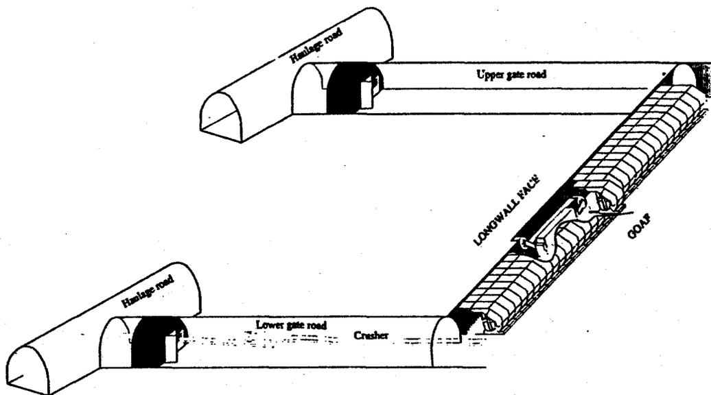
Figure 2: Diagram of a mechanized retreating longwall face
