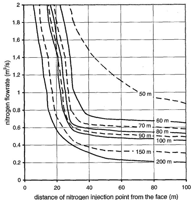
Figure 5. Optimization of Nitrogen Injection (Each Line Shows the Position of the 1% O<sub>2</sub> Fringe in the Goaf for Given Flowrates and Locations of Injection; Figures Indicate the Distance of this Fringe From the Face Line)
