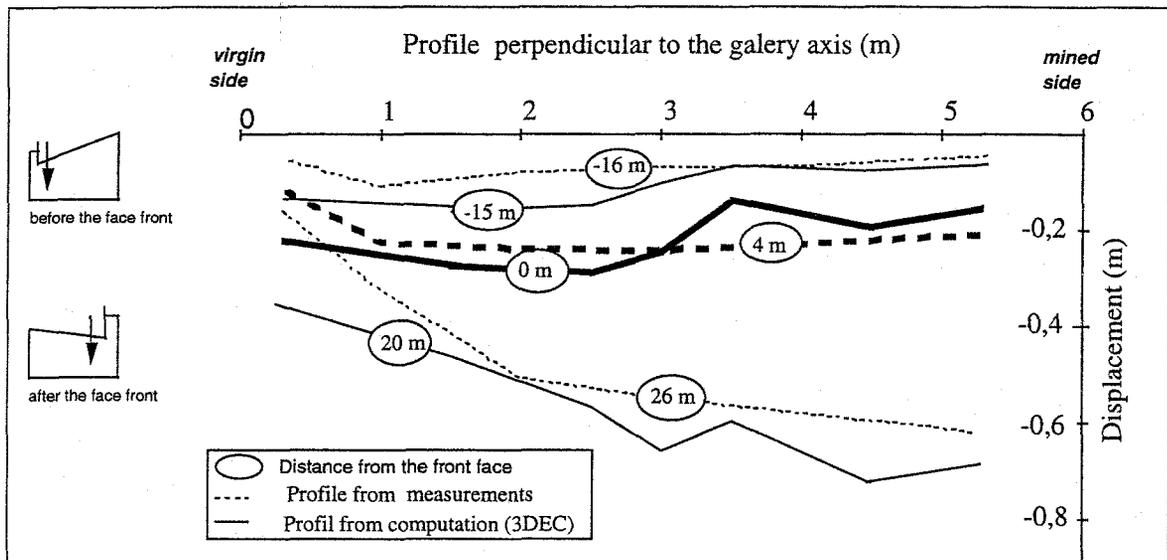
Fig. 6 : Evolution of the gallery roof deformation
