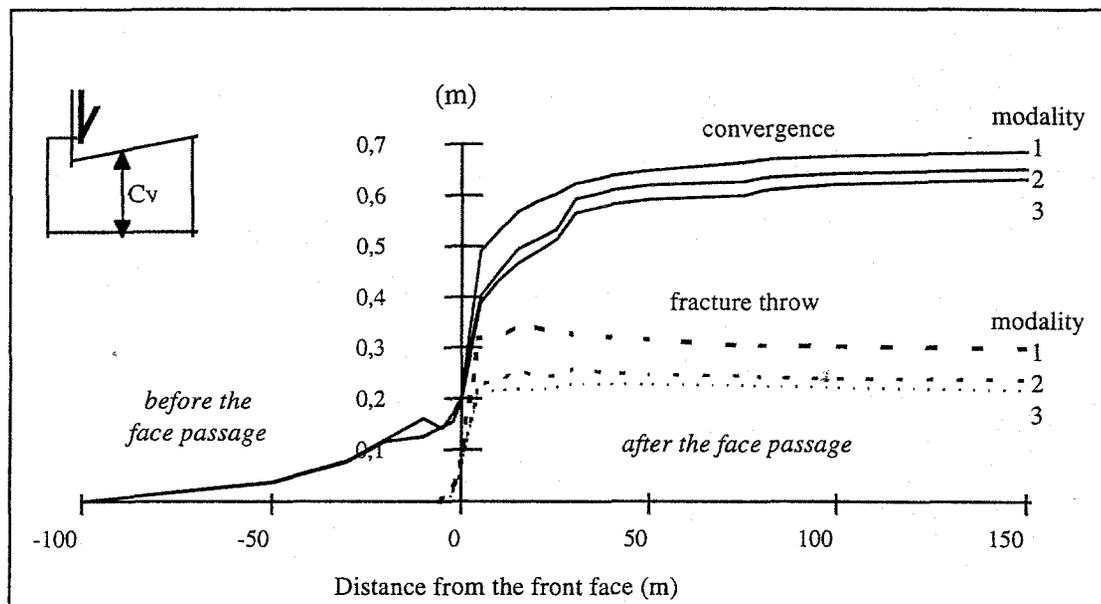
Fig. 11 : Roof displacement for the three modalities
