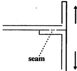
Figure 1: Peel test
