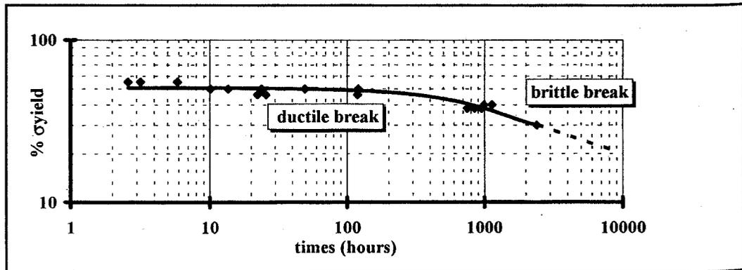
Figure 5: Stress cracking
