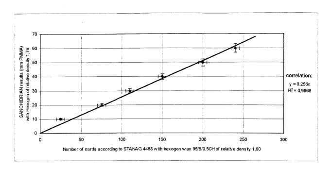
It can be seen that practically the same curve is obtained in both cases (see the coefficients of the equations of the lines given on the curves). It can be concluded from these correlations that there is equivalence between the two methods, and the following correspondence can be deduced:
