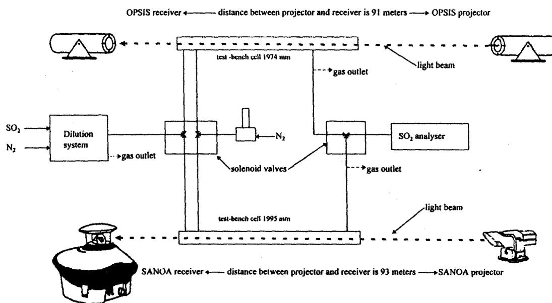
Figure 2 : test-bench for  $\text{SO}_2$  set up in tunnel
