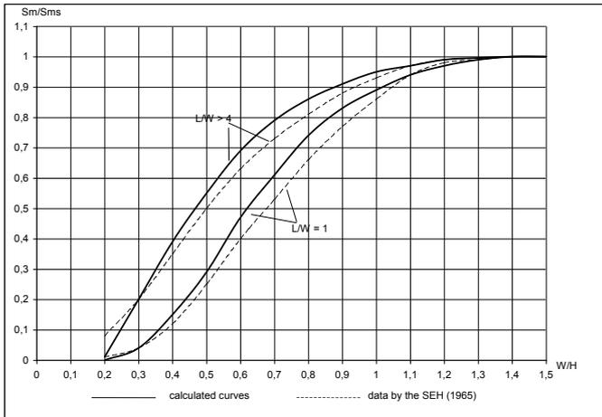
Fig. 1. Dependence of the maximum subsidence on  $W/H$
