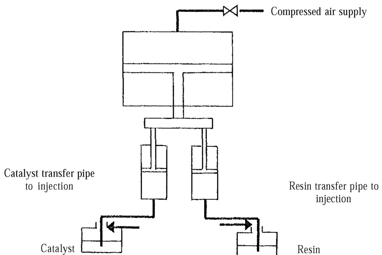
Figure 3. Operating principle of an injection pump
