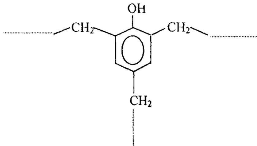
Figure 2. Three-dimensional lattice produced by phenol-formol polycondensation
