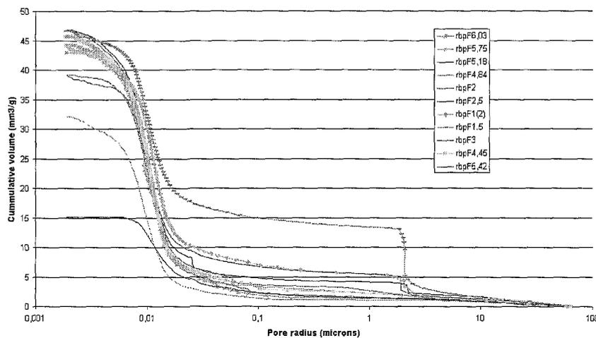
Fig. 4 : Mercury injection curve for humidity steps reach from drying after fast wetting realised on dry samples
