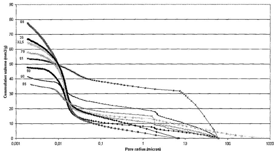
Fig. 5 : Mercury injection curves on wet samples
