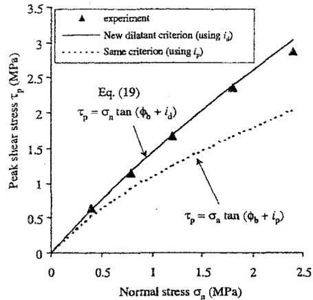
Fig. 7. Shear strength predicted by the new dilatant shear strength criterion when using dilatancy angle ( $i_p$ ) and the new proposed dilatancy-degradation angle ( $i_d$ ) and compared to the experimental results for the natural schist joint mortar replica.
