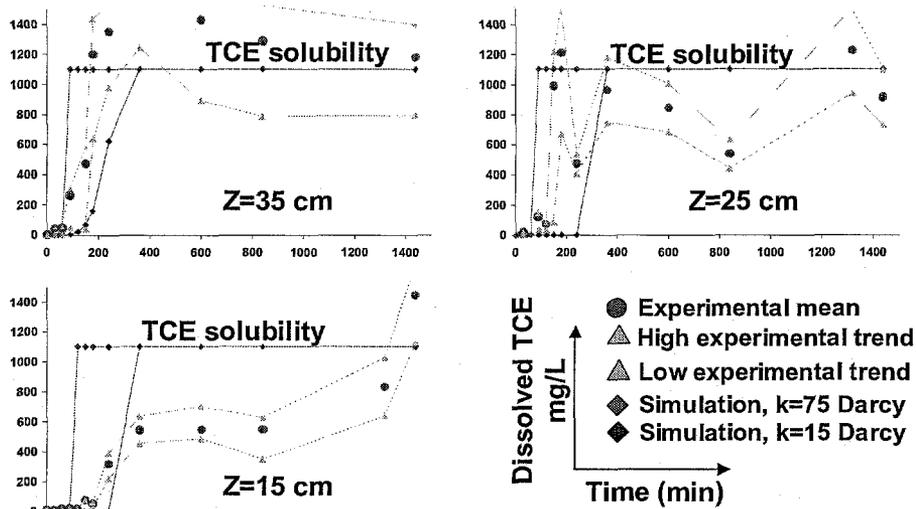
Figure 4: Calculated and experimental evolution of dissolved TCE concentration.
