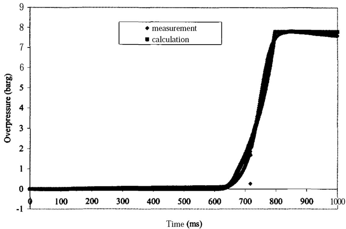
Figure 3: comparison between calculated and measured pressure evolution inside the closed ISO 1 m<sup>3</sup> vessel for a starch dust air explosion
