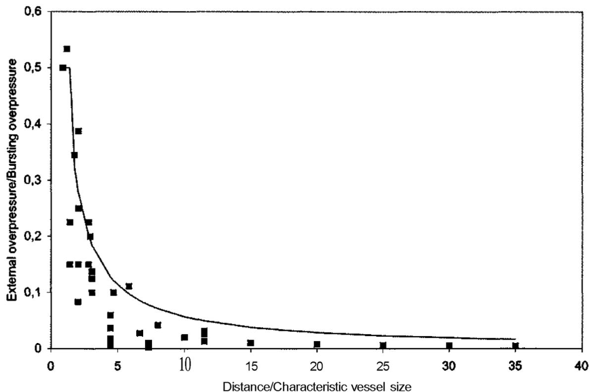
Figure 8: predicted (curve) and measured (squares) external overpressure
