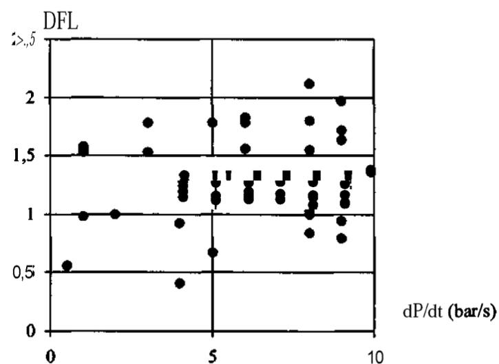
Figure 6: Dynamic load factor ( $DFL = \text{dynamic bursting overpressure}/\text{static}$ ) measured for thin aluminium membranes ( $0,5 \text{ m}^2$ ) submitted to dust explosions of various violences
