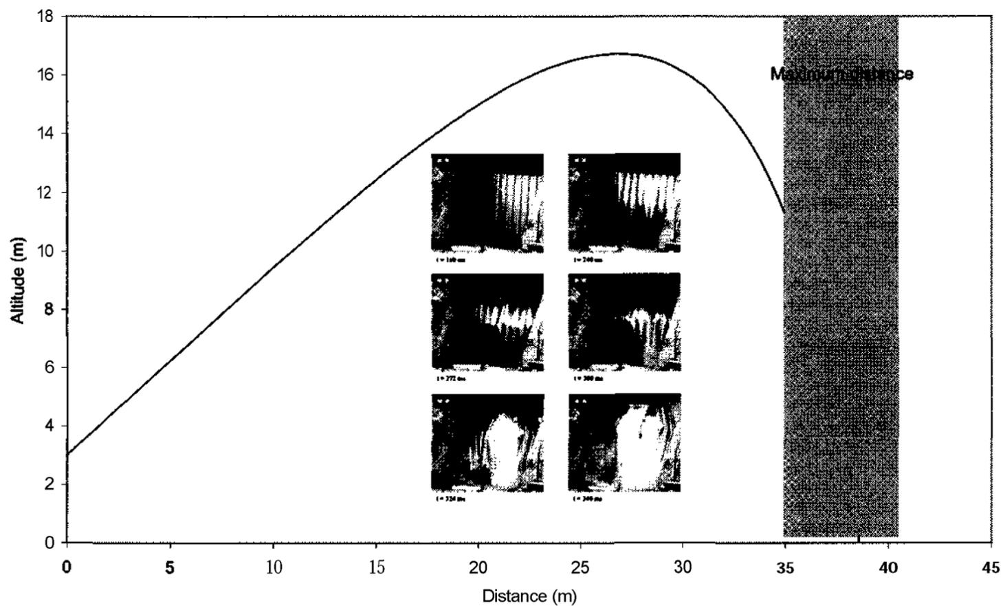
*Figure 7: bursting of a  $10\text{ m}^2$  steel panel wall submitted to a  $100\text{ m}^3$  starch dust explosion and projection of debris (curve = prediction ; grey zone = max. observed throw distance)*
