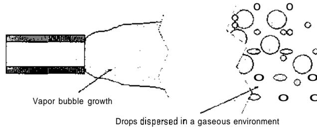
**Figure 1 : Schematic diagram of a two-phase jet**
