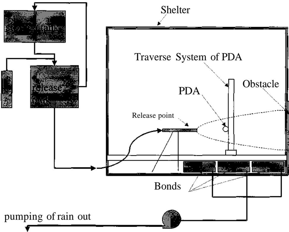
Figure 4 : Diagram of the experimental set-up
