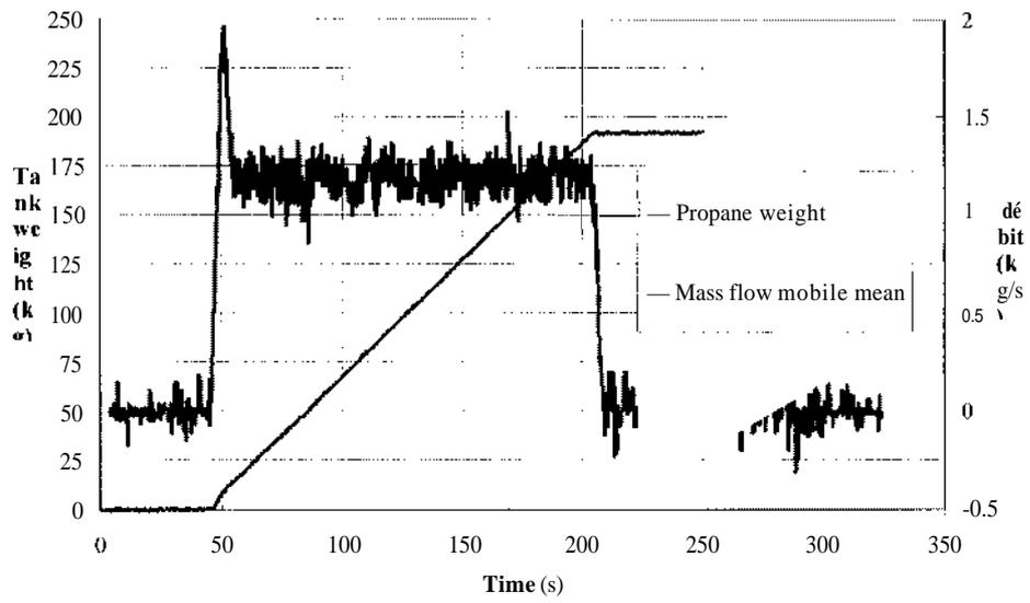
Figure 9 : released mass flow and propane weight
