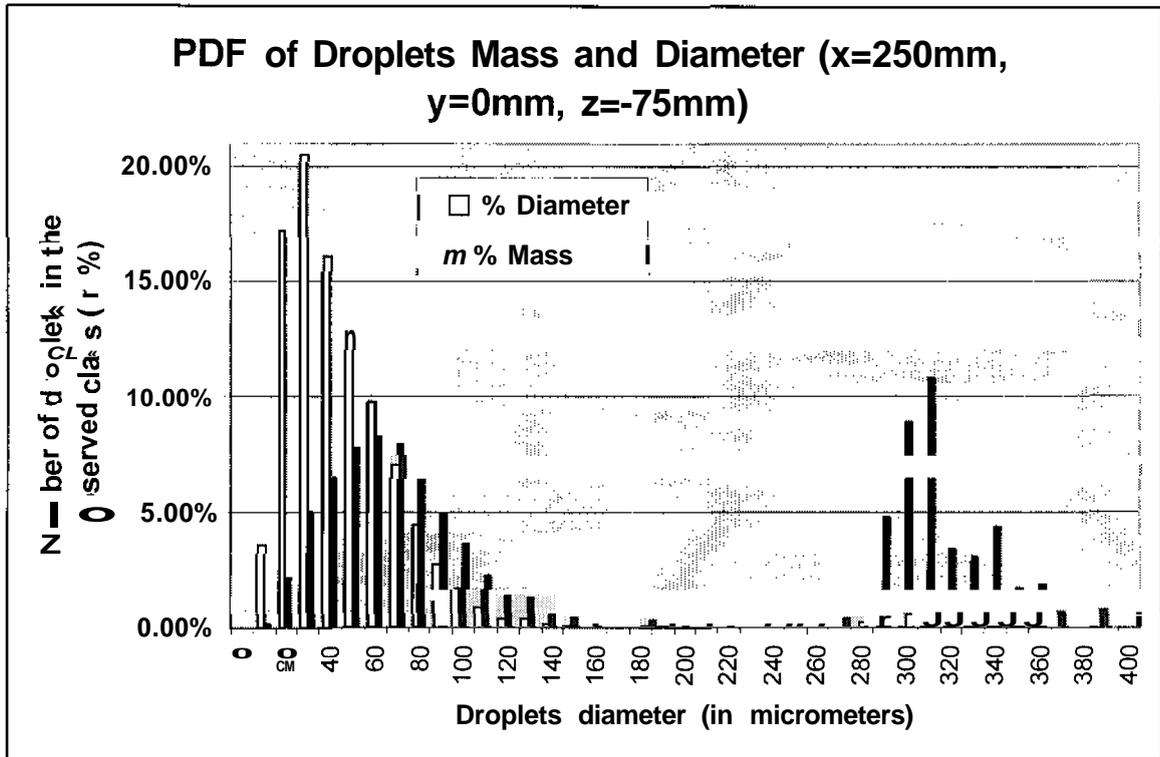
Figure 7 : Number of droplets in the observed class (in %) versus droplet diameter for a free jet of propane at 7.5 bar through an orifice diameter of 25 mm
