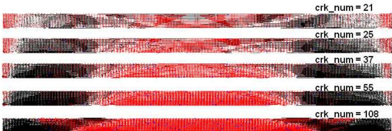
Figure 7. Bond forces in the cement between particles (black = compression, red = in tension) of the PFC inclusion at (from top to bottom)  $\lambda = 0.5, 0.4, 0.3, 0.2$  and  $0.1$ . Tensile cracks are shown in blue.
