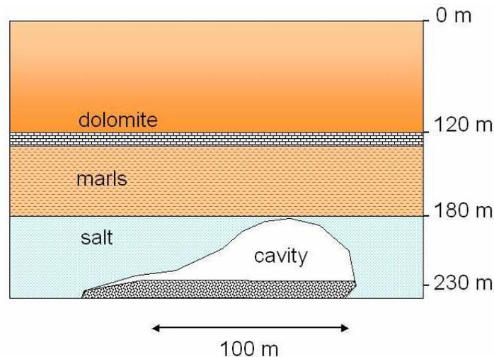
Figure 1. Schematic section of the salt cavity and main geological facies.
