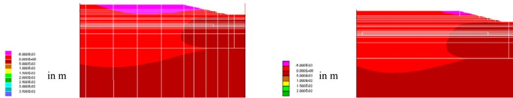
Figure 15: Horizontal displacement in fractured and unfractured medium
