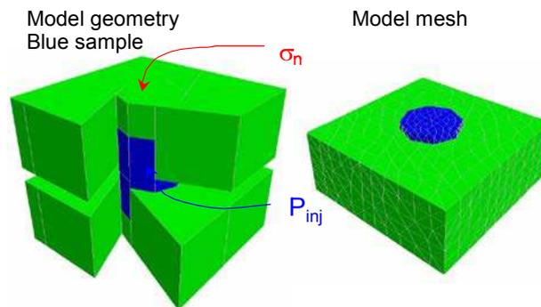
Figure 9: 3DEC model used for test interpretations
