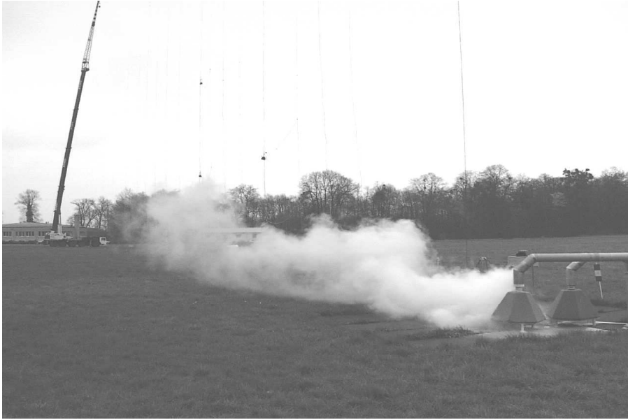
Figure 2. View of a part of the experimental arrangement showing the spill point and vertical steel ropes
