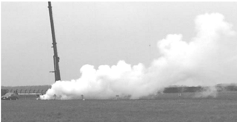
Figure 3. Example of a liquid helium cloud (test 7)
