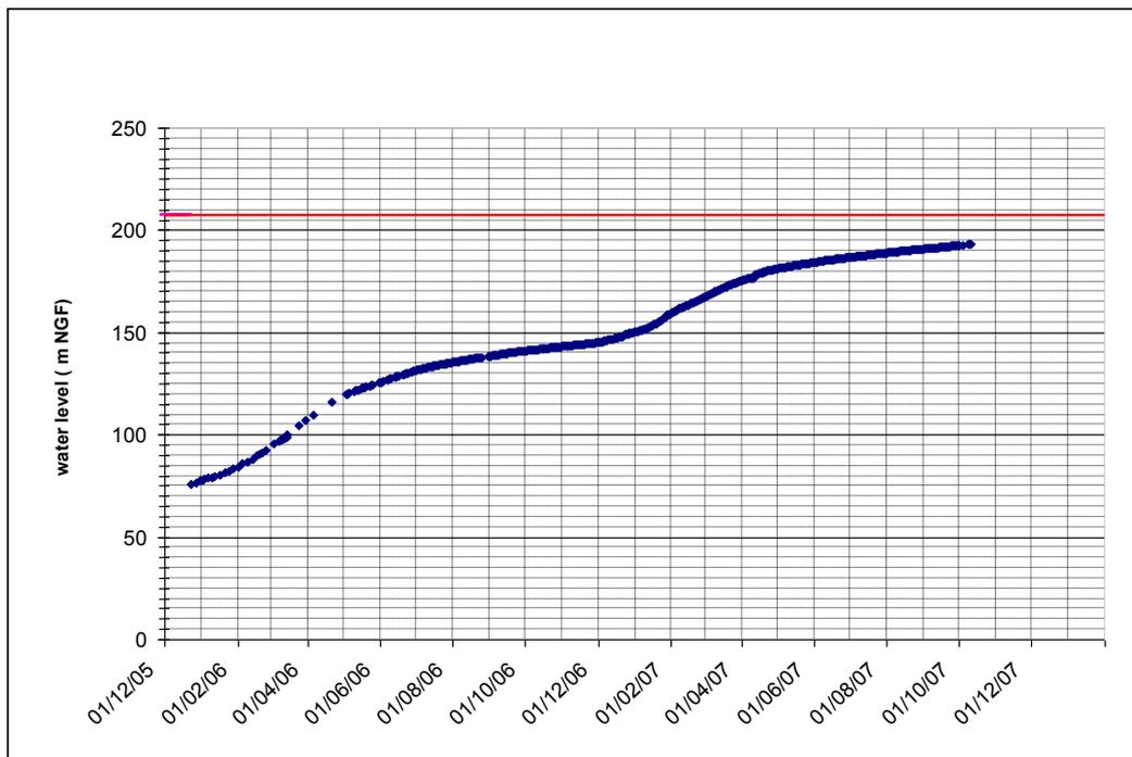
Figure 3. Water level evolution in north iron basin
