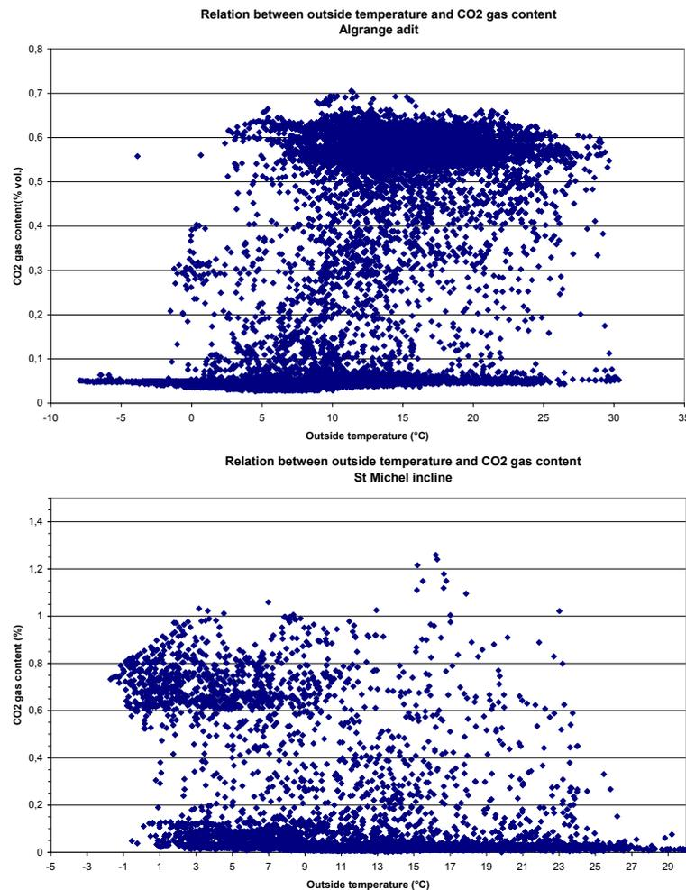
Figure 6. Relation between temperature and CO<sub>2</sub> gas content
