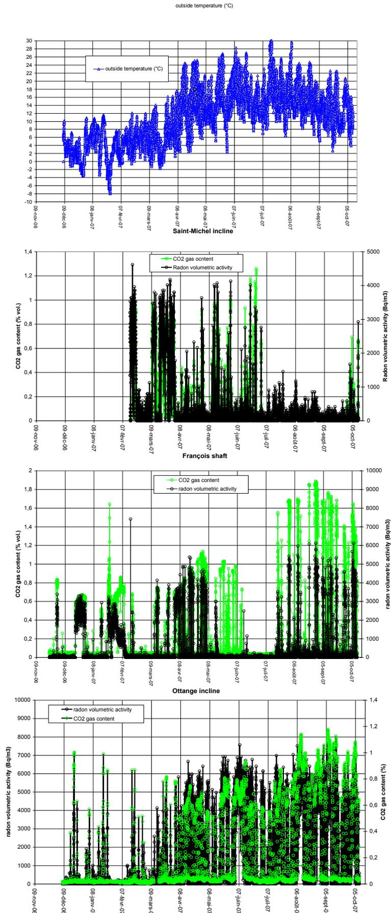
Figure 5. Volumetric activity of radon and CO<sub>2</sub> gas content measured at different openings of north iron basin
