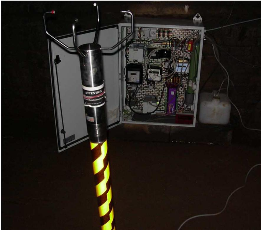
Photo 1. Measuring station and anemometer in Algrange adit
