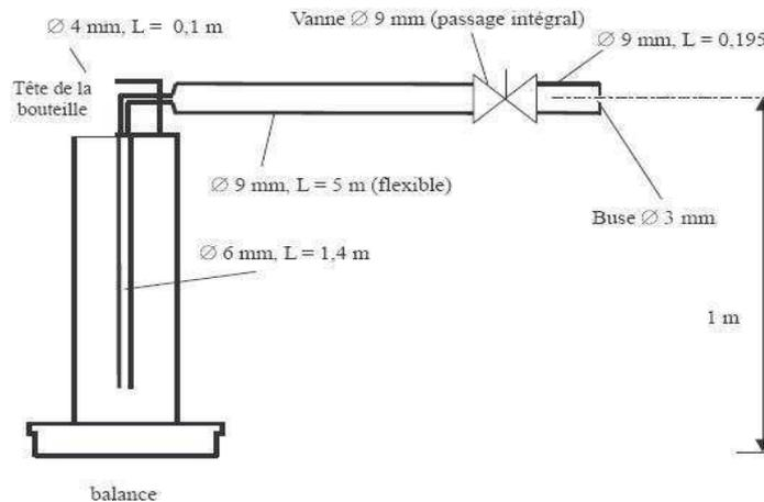
Figure 2 : schematic representation of the discharge device
