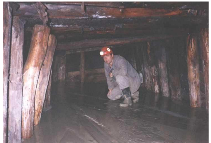
Figure 5: Injected paste in an abandoned Slovenian Mercury mine (By courtesy of Bojan Režun).
