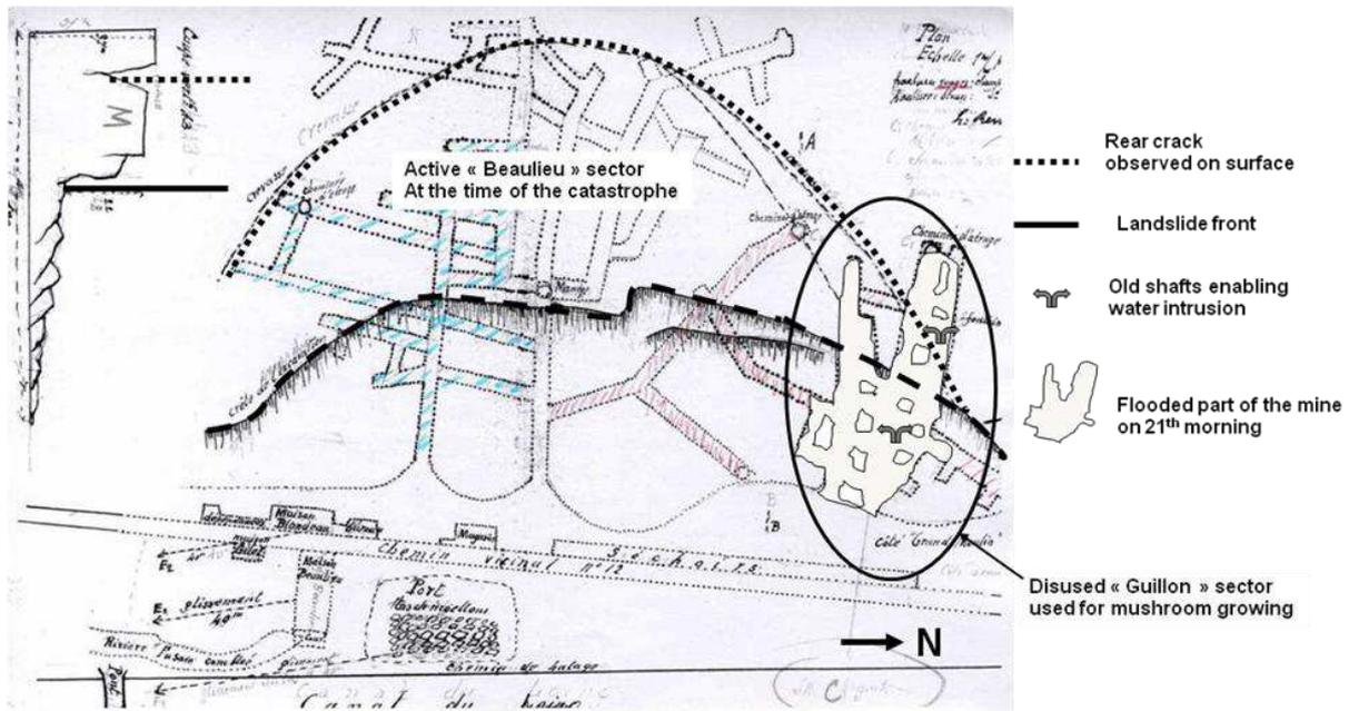
Figure 6: Schematic view of the collapse and associate landslide of the Lorry hillside on January 21<sup>th</sup>, 1910.
