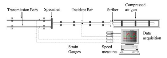
Figure 1. SHPB bending test set-up
