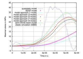
Figure 9:  $\sigma(t)$  estimated using the incident experimental wave and the simulated reflected waves.
