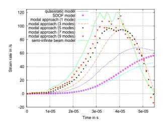
Figure 11:  $\dot{\varepsilon}(t)$  estimated using the incident wave measured and reflected waves obtained by the various elastic models.
