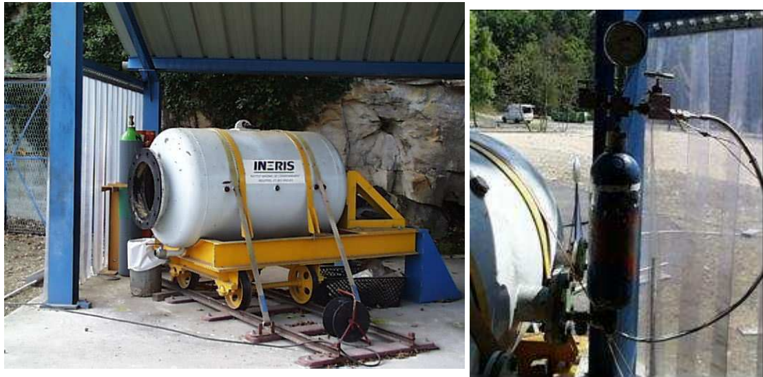
Figure 1 : sketch (dimensions in mm) and views of the 1 m 3 vessel (injection device of the fuel on the right picture)
