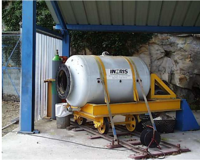
Figure 1 : sketch (dimensions in mm) and views of the 1 m 3 vessel (injection device of the fuel on the right picture)
