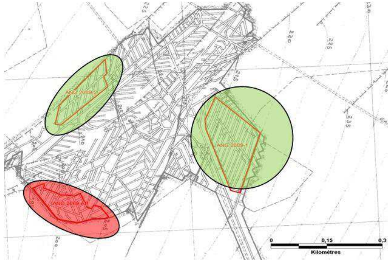
Figure 1: in red, example of failed sector that has caused a surface disruption; in green, nearby sectors in which the pillar dimensions predict stability.
