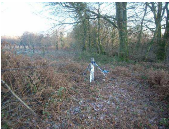
Photos 7 and 8 - Inspection of an inclined shaft through a 125 mm diameter borehole, the distance between the winder (in the van) and the tripod is about 80 m.
