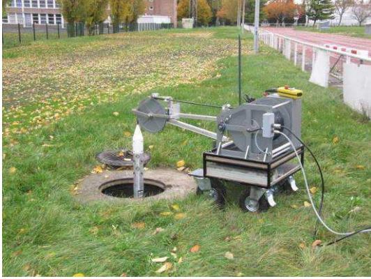
Photos 3 and 4: two examples of inspection of a shaft directly from the winder on its wheels
