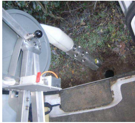
Photo 6 - inspection of a cavity through a 140 mm diameter tubed borehole directly from the van
