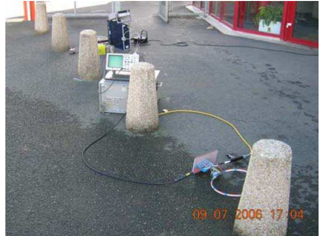
Figure 4. On site testing for a magnetic field sensor
