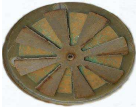
Figure 1. Corrosion marks of the rotating part as well as fix part. Note that blades are damaged.
