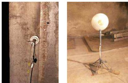
Figure 3: Blast pressure gauge
