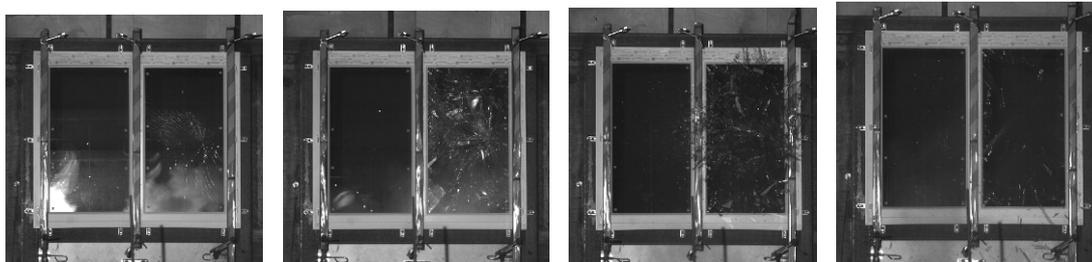
Figure 8: Insulating glass subjected to a blast wave
