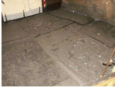
Figure 9: Fragments landed on the floor – zone 0-3 m
