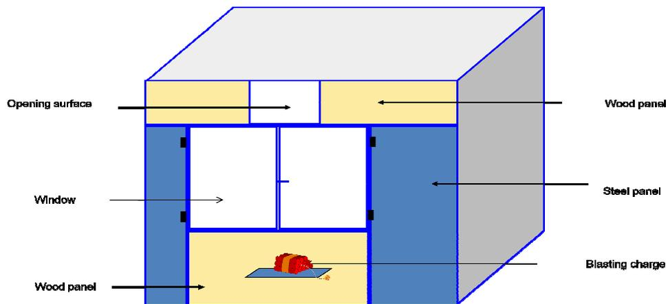
Figure 2: Schema of experimental device
