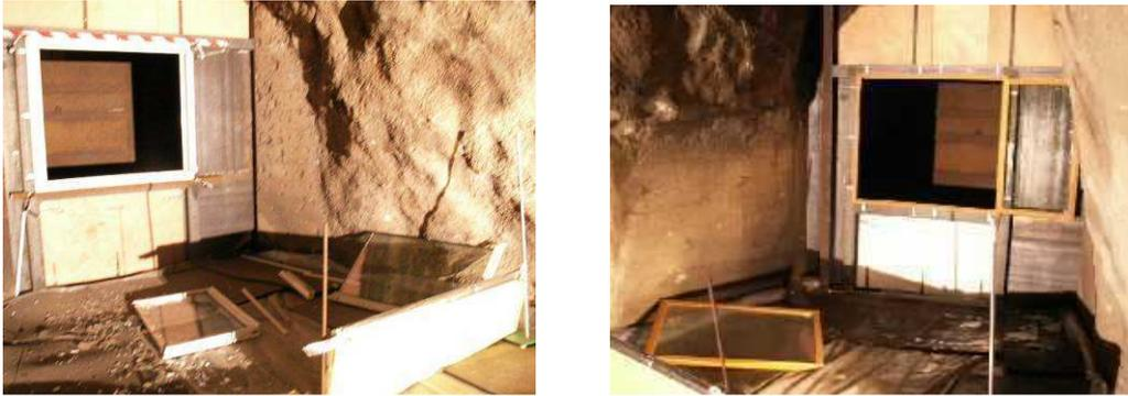
Figure 15: Projection of mofile frame of French style inwards opening window composed with PVC frame (at left) or wood frame (at right) and a common locking system (catch and strike)
