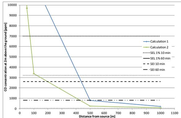
Figure 2 : calculated concentration of CO at 50 m, 100 m, 500 m for two calculations of the first test case ; SEL 10 min stands for *Seuil effet irreversible* is the threshold of irreversible effects for 10 min exposure; SEL 1% stands for *Seuil effet létal* is the threshold of first lethal effects above which 1% mortality can be observed in the exposed population
