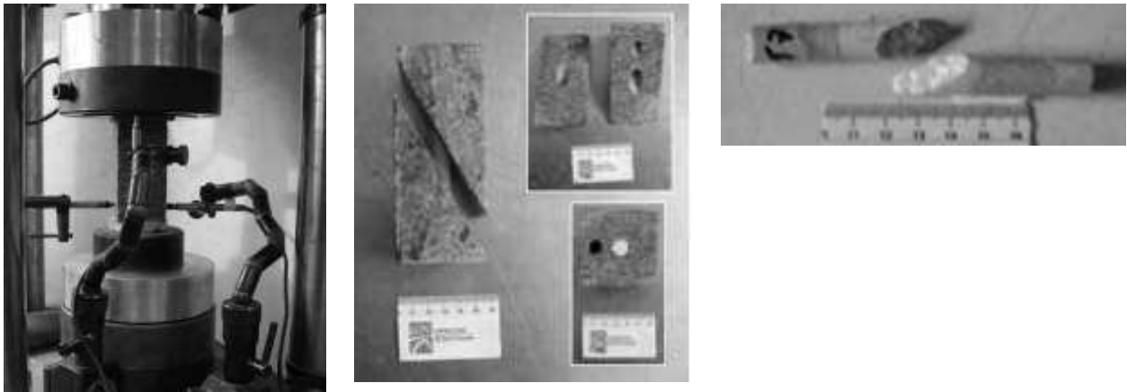
Figure 8: Picture of the uniaxial cell used for the experiment “alteration quasi-static” (left). Sample in the granite base (middle) and the broken sample after the test (right) (after Druon).
