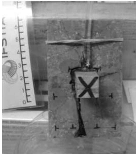
Figure 14: Picture of Montagnole limestone ( \text{CaCO}_3 ) sample surface degradation by acidic solution ( \text{H}_2\text{O} ; \text{H}_2\text{SO}_4 )
