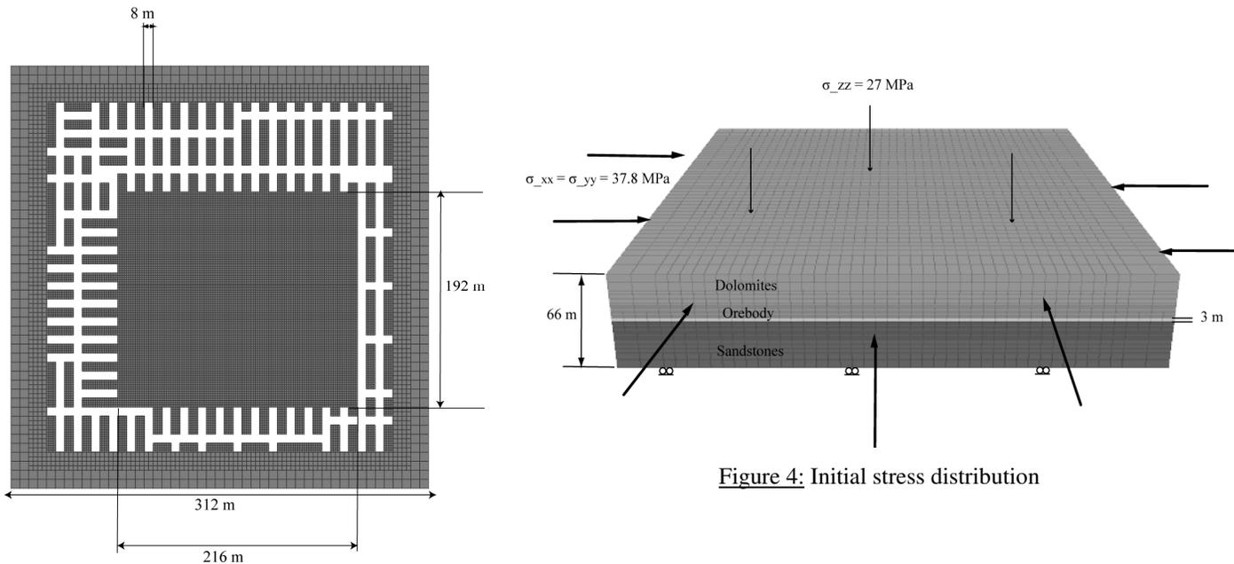
**Figure 3:** Horizontal view and dimensions of the model
