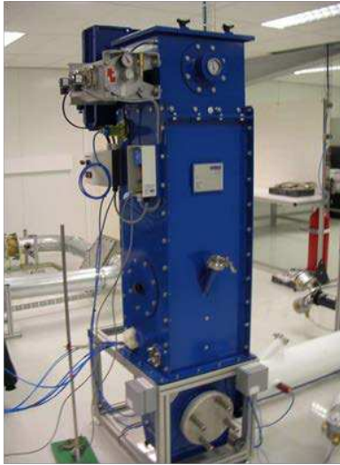
Figure 3: Purposely built dust collector
