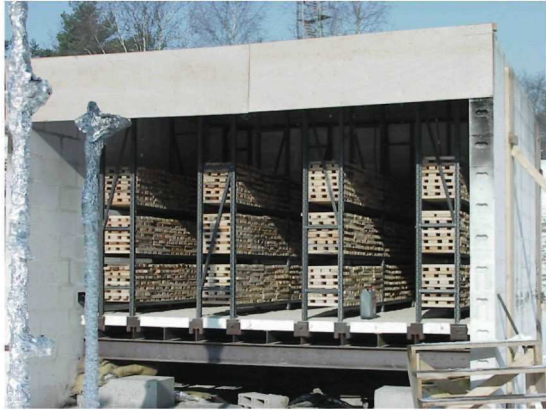
Figure 1. Picture of the experimental set-up (of the 3-tier, highly compact storage with a low containment level)
