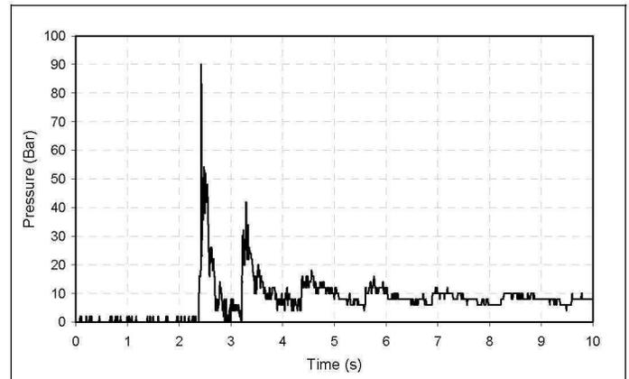
Figure 2: Pressure-Time History - Detonation-( $P_i=1.2$  bar)
