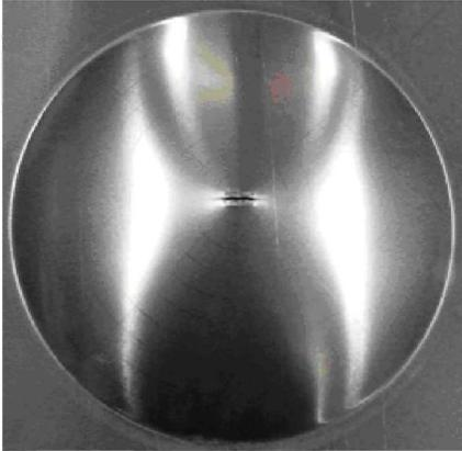
**Photo 4: Experimental Result for Al5754 Notched Plate**
