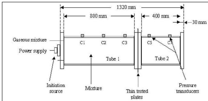
Figure 1: Experimental Device
