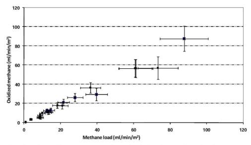
Figure 8. Oxidized methane fluxes versus methane loads for the site B with relative errors bars
