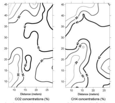
Figure 3. Methane and carbon dioxide concentrations of the gas probe for the site A
