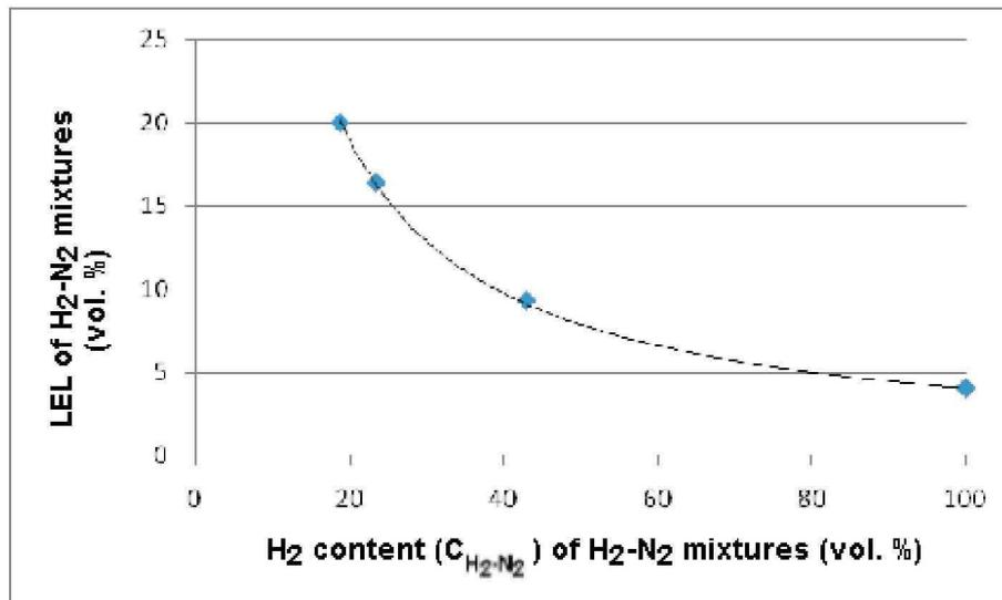
Fig. 2 : LEL variation of H<sub>2</sub>-N<sub>2</sub> mixtures versus their H<sub>2</sub> content C<sub>H<sub>2</sub>-N<sub>2</sub></sub>
