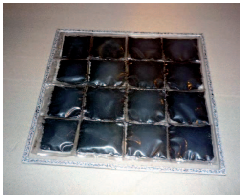
Fig. 3. The resulting small-scale structure model composed of a hollow slab and small bags of lead powder representing the load.
